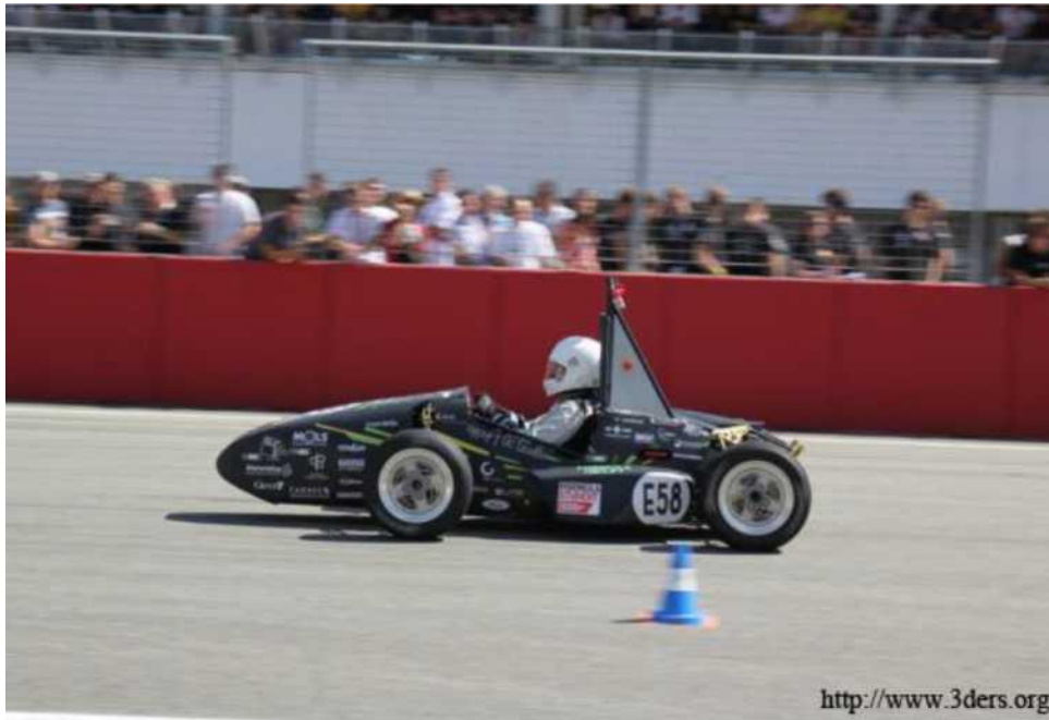
The first 3D printed racing car reached a speed of 140 km/h. Acceleration from 0 to 100 km / h - in 4 seconds.
