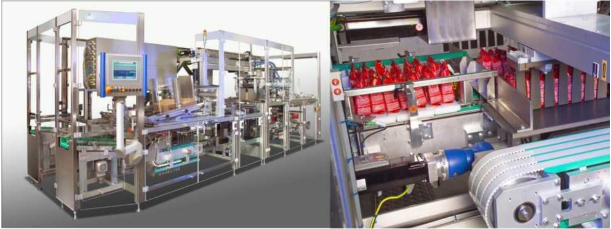
For example, this GPS produces 100 bags per 125 rproduct per minute.
