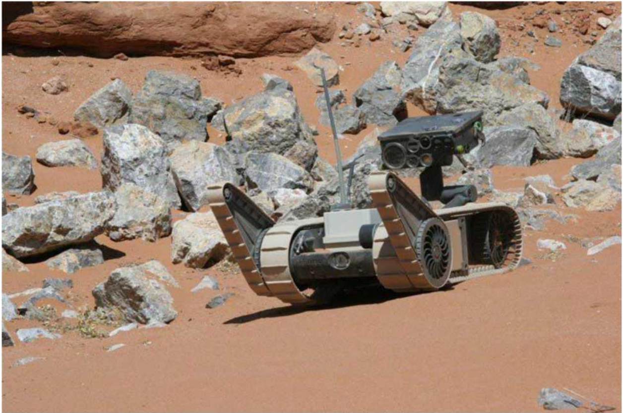
For example, the XM1216 reconnaissance robot for ground operations.
